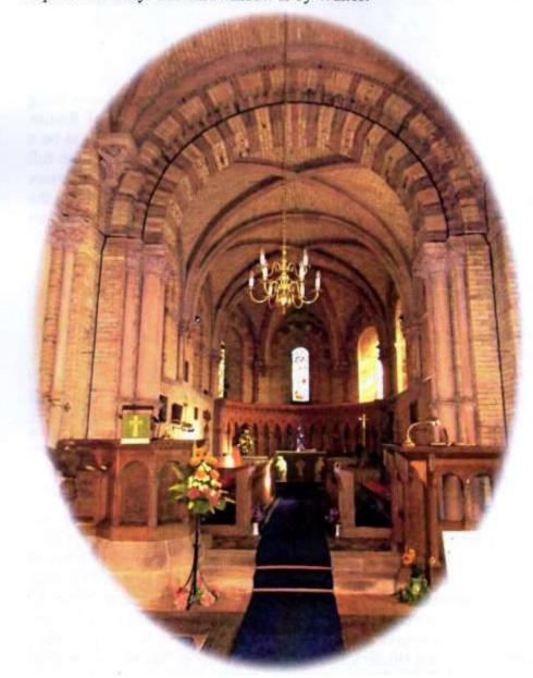
Victorian brickwork is unsurpassed in quality, exemplified here by the specially moulded bricks to frame the windows, with elongated wedge shaped bricks to form the arches over the windows, also to construct the main arches at the crossing under the tower, and to form the ribbed vault ceiling.
